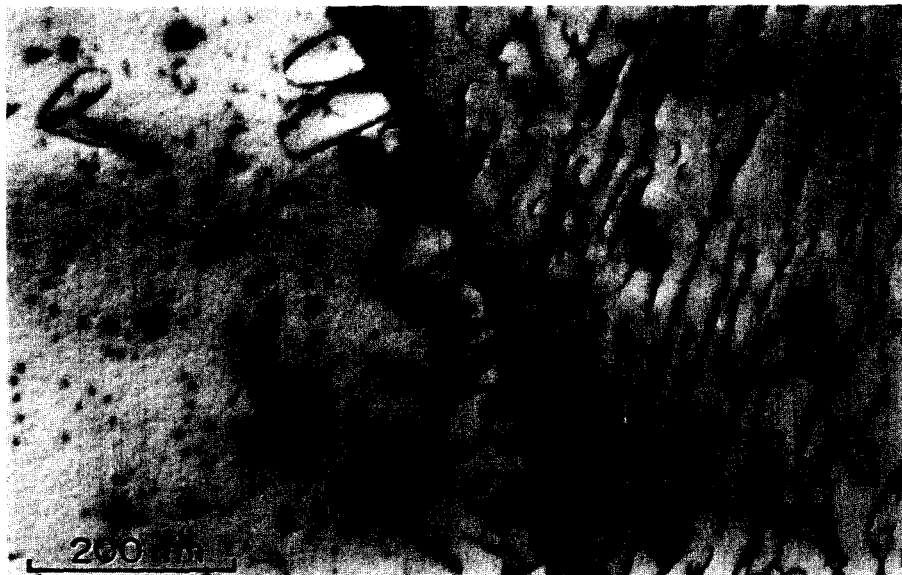
Fig. 6. Difference in dislocation and void structures between two adjacent grains in a thin foil of Ni-2 at.% Cu irradiated with fission neutron to a fluence of 9 \times 10^{23} n/m 2 (> 1 MeV) at 673 K.
